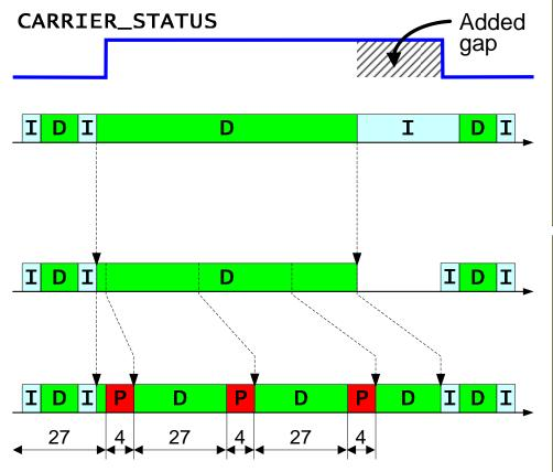
1. By controlling CARRIER\_STATUS signal, the RS precisely increases the gap between frames to accommodate the FEC parity.
