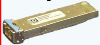
XFP/ QSFP 75mm L x 18 mm W x +9mm H
