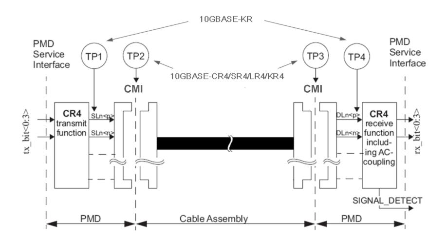
10GBASE-CRN/SRN/LRN/KRN Link Diagram (half link is shown)
