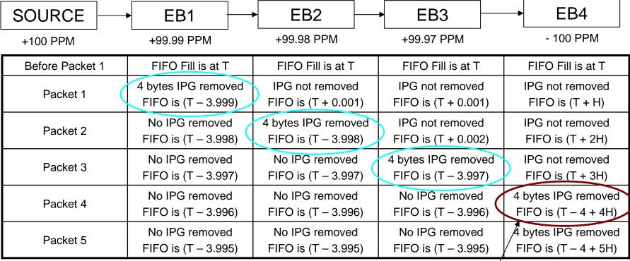
Using this example we can see that the maximum storage needed at the last Elastic Buffer is N \* H bytes just before the adjustment.
