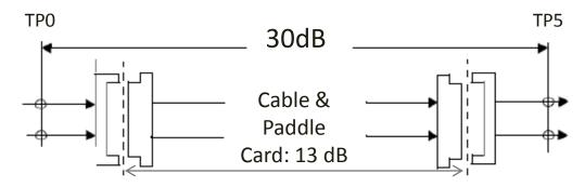
3.5 m cable assembly link budget example with 8.5 dB host loss: 30 dB @12.89 GHz (FEC not Required)
