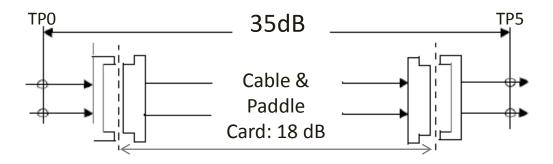
5 m cable assembly link budget example with 8.5 dB host loss: 35 dB @12.89 GHz (FEC Required)
