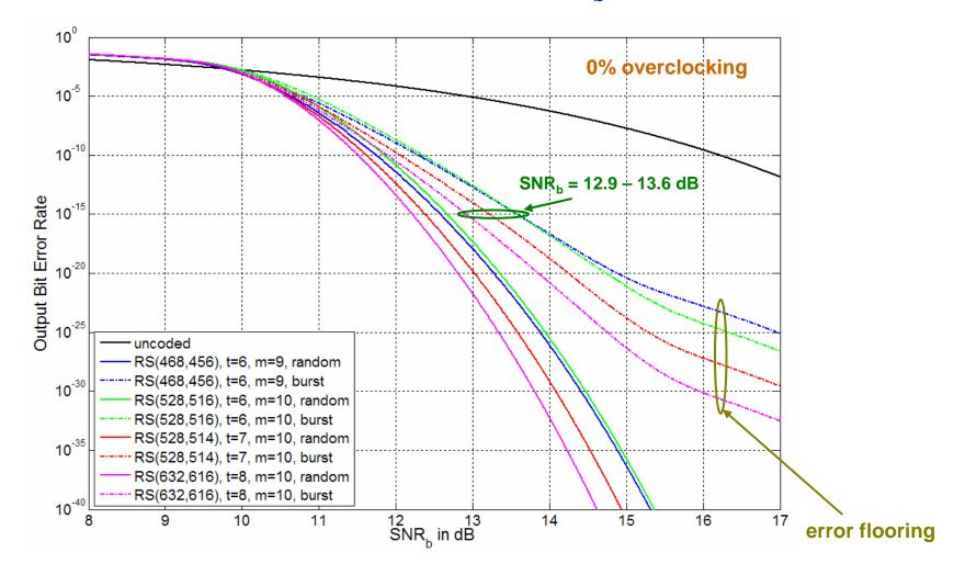
For 0% overclocking and  $6 \le t \le 8$ , SNR<sub>b</sub> at DFE slicer input must be 12.9 - 13.6 dB to achieve target bit error rate 1e-15
