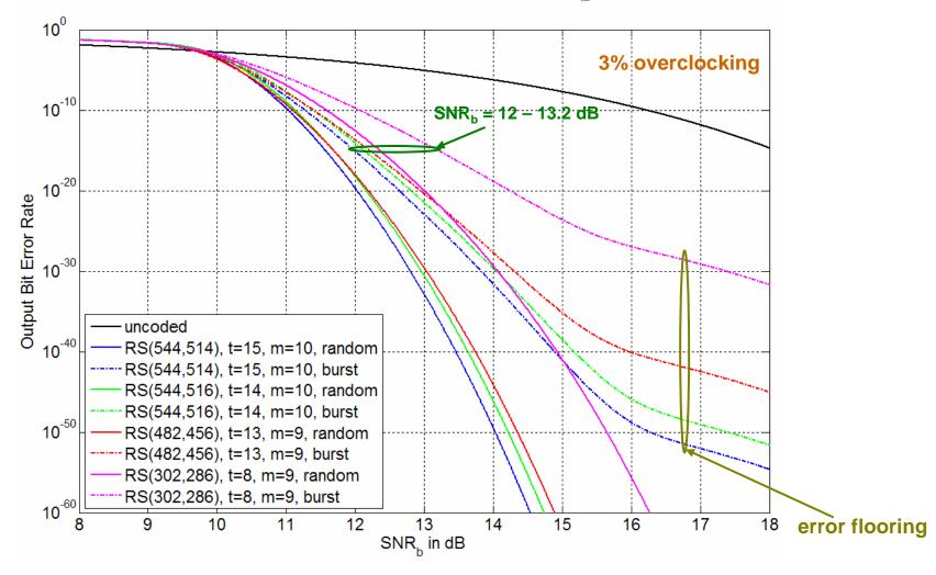
For 3% overclocking and  $8 \le t \le 15$ , SNR<sub>b</sub> is in the range 12 - 13.2 dB to achieve target bit error rate 1e-15
