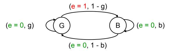
■ DFE slicer bit error probability w/o error propagation  $p_{sl} = (1-b) p_{bl}$
