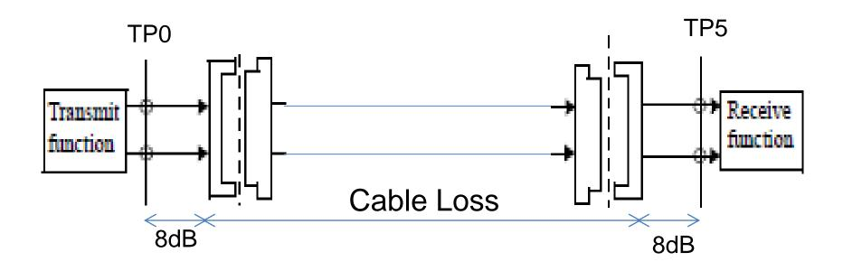
30dB without FEC Allows Cable loss of 14dB ie 3m AWG26
