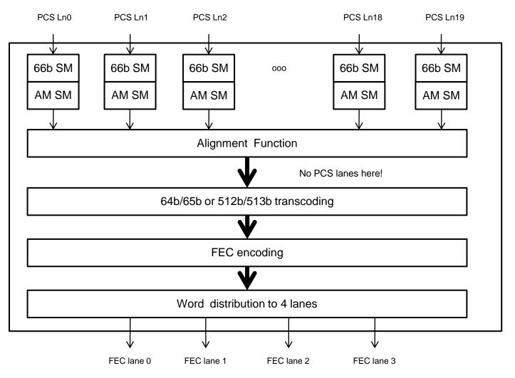
Below shows the processing for the FEC options that have been proposed so far (RX side processing):
