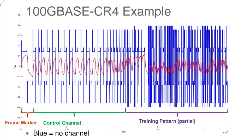
Red = after IL = ~33dB @ 13GHz channel (with 'INITIALIZE' TXFFE equalization)
