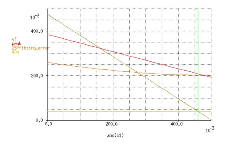
SNDR due to fitting error only is falling off a cliff, and below 15dB when  $v_f$  reaches 40mV (green line). If we use pulse peak as a reference it hold up much better.
