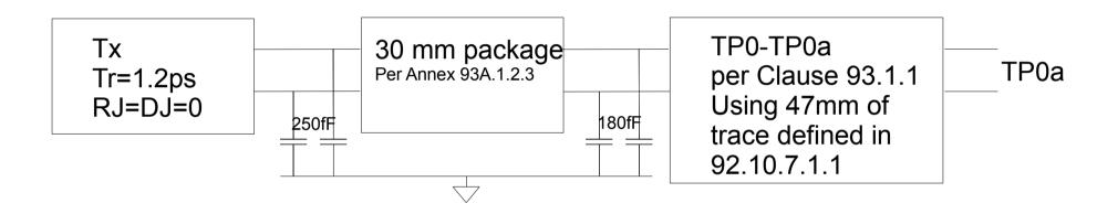
I used the above channel as a model of the COM reference transmitter
