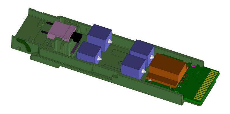
The above figure shows that four, single laser TOSAs and a quad photodiode ROSA can fit within the QSFP28 space with sufficient room for the electronics. This is a possible approach for implementation of a 100G PSM4 based on directly modulated DFB lasers.
