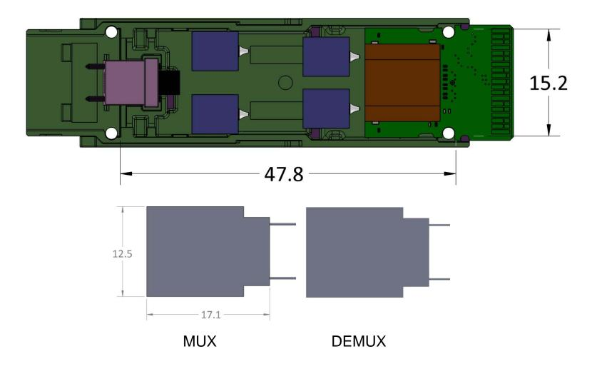
The above figure shows that while the individual TOSAs and ROSA from the previous page may fit, there's insufficient room to add commercially available MUX & DMUX devices.
