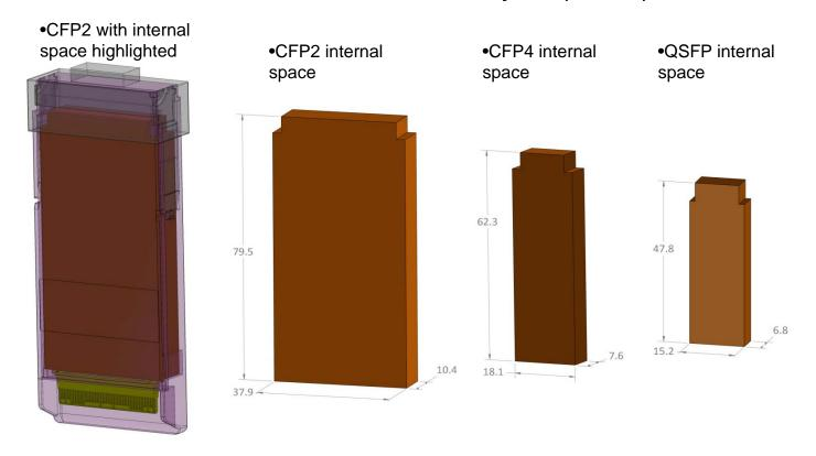
Among the possible form factors for 100G (4 x 25G lanes) transceiver modules are CFP2, CFP4 and QSFP28. The above figure shows the internal space available for the transceivers. The smallest and most challenging is QSFP28.
