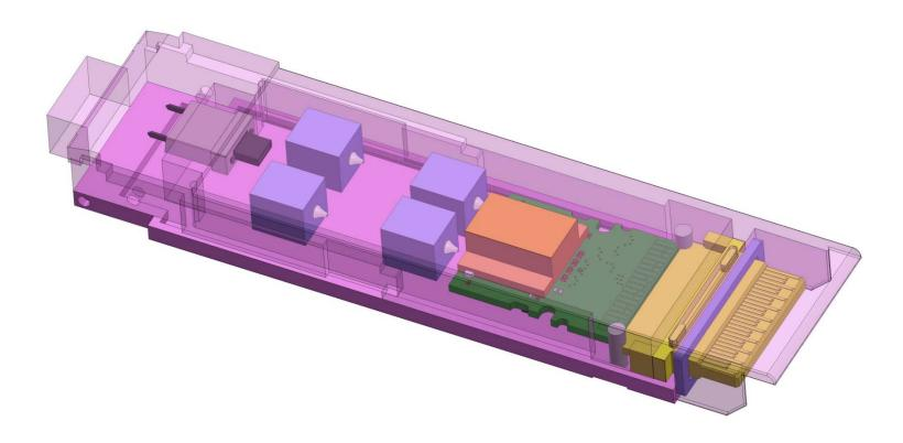
The above figure shows the device layout from the previous pages within the space of a CFP4. Again, there appears insufficient room for commercially available MUX & DMUX devices and more compact solutions will be needed. For 100G LR4 one approach is expected to be a monolithic Directly Modulated (DM) DFB array integrated with the MUX.
