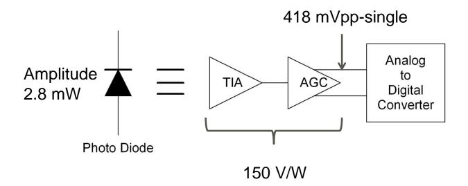
Input amplitude for ADC should be controlled around 400 mVpp-single. For this operation, AGC should be required for receiver.
