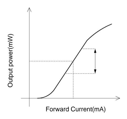
Driving voltage was limited for linear operation of commercial DMLs. Characteristic enhanced DML can improve power budget.
