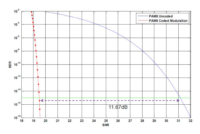
• PAM8 coded modulation FEC delivers 11.67dB coding gain
