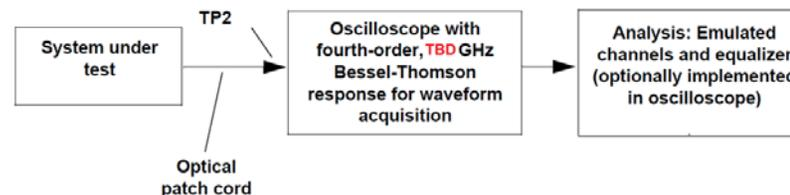
Figure 96-5—Transmitter test fixture and test points
