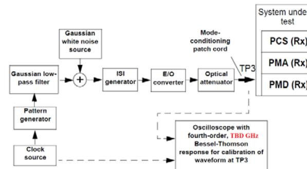
Figure 96-8— Reference measurement configuration for comprehensive stressed receiver sensitivity and overload test
