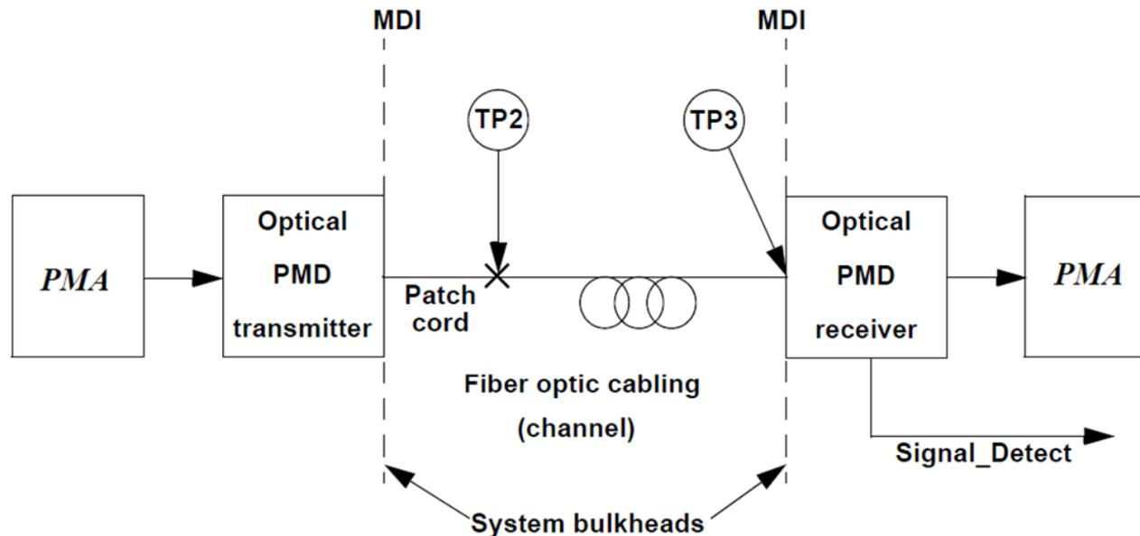
Figure 96-4—PMD link Block diagram
