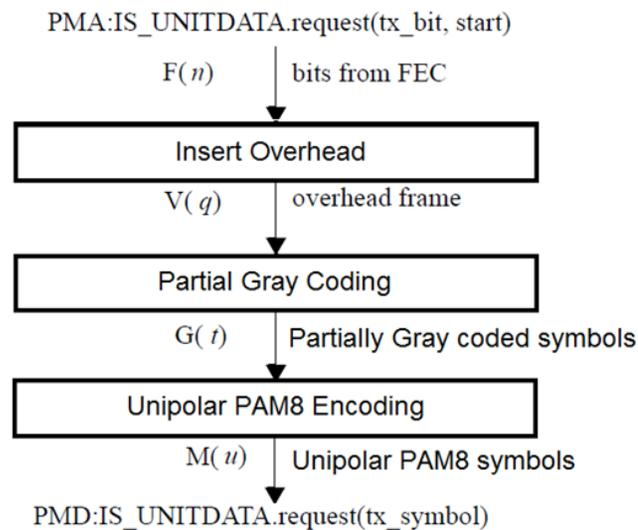
Figure 96–2—Transmit adaptation process diagram
