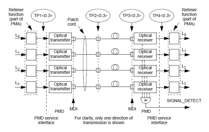
TP1 and TP4 are reference points for the CPPI-4 electrical interface specifications
