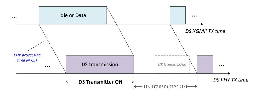
The TDD cycle timeline is propagated from MAC Control to PHY at CLT start
