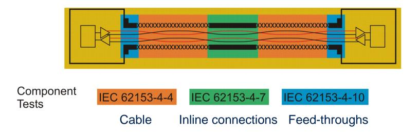
Triaxial tube allows measuring screening properties of individual components along the channel
