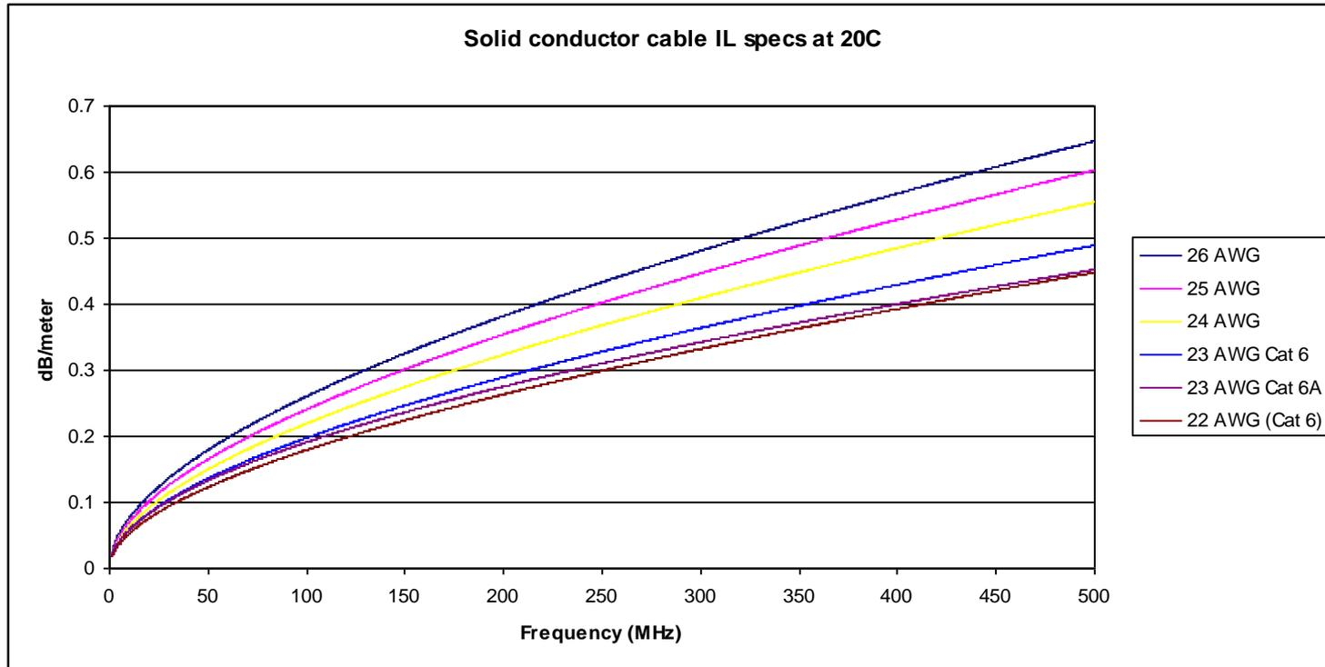
**Solid conductor cable IL @ 20C (dB/meter)**
