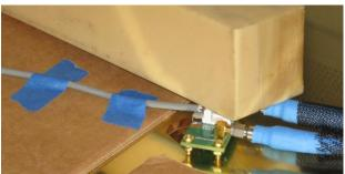
This mounting configuration supports the more recent standards discussions about cables tested closer to the reference ground plane
