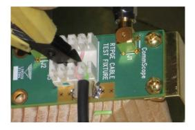
Side mount brass stands position the terminations for conventional stripline cable height over ground plane
