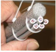
Here, the "center" one could be the 3 meter extended channel, and placing it centered against the tube allows all four other channels consistent direct coupling
