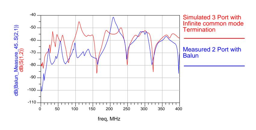
Mode Conversion vs. Impedance Variation (6dB difference of peak value, simulations from 3-port BCI S-parameter measurements)
