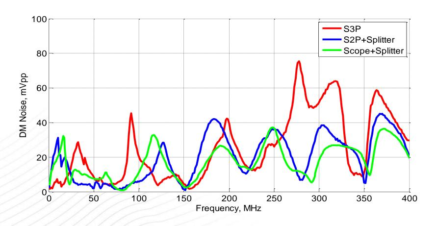
Notes: VNA and Scope measurements are close when using a differential splitter. Larger resonances are seen using 3-port VNA measurements
