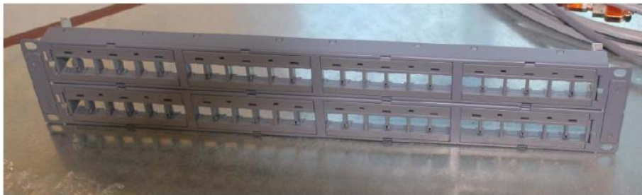
A panel for mounting jacks
