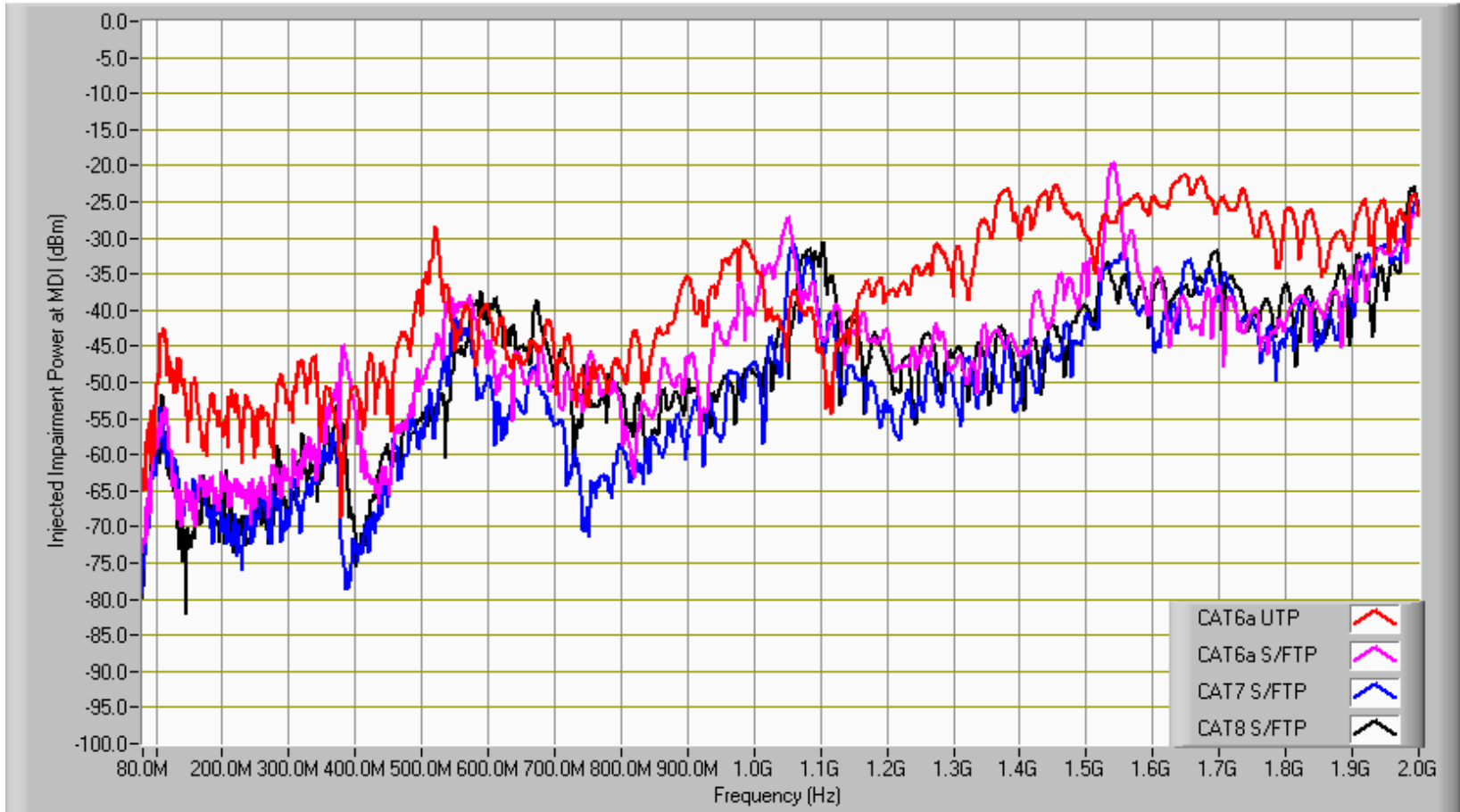
common-mode noise @ MDI, cable comparison, ~6dBm input
