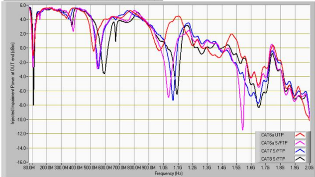
cable clamp power @ DUT end, constant 6dBm source input
