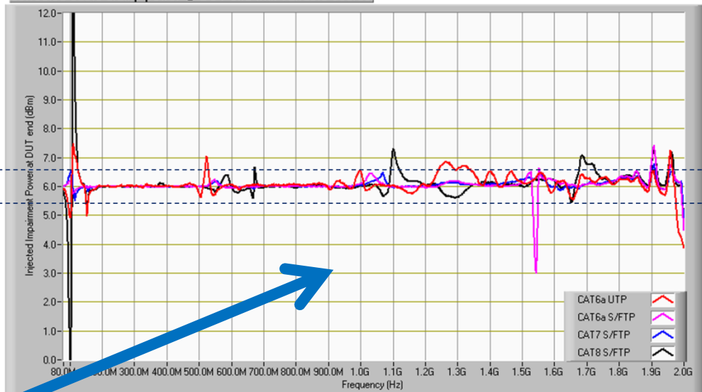
corrected cable clamp power @ DUT end with variable source
