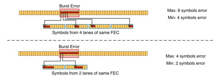
Only orthogonal interleaving will reduce the error probability on each FEC;
