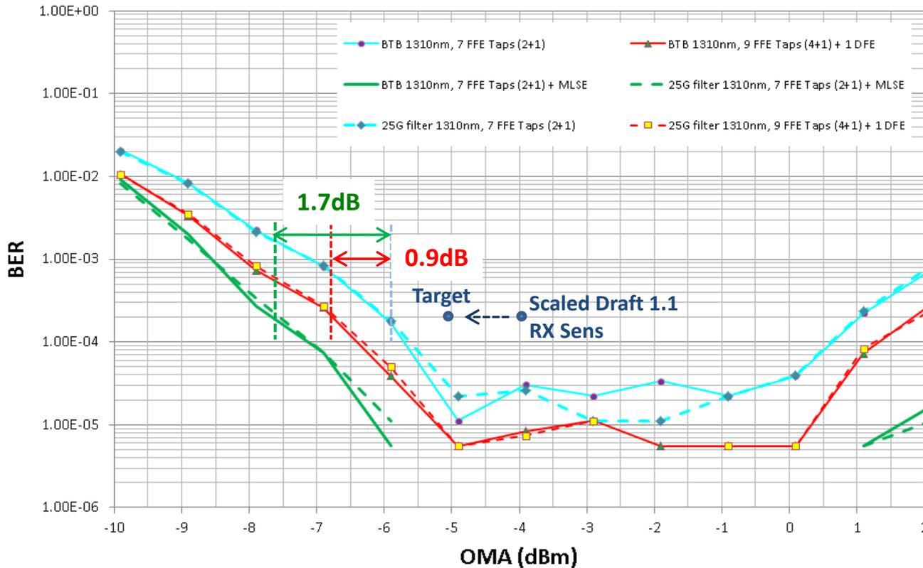
25GHz BW filter used, to simulate more restricted BW components.
