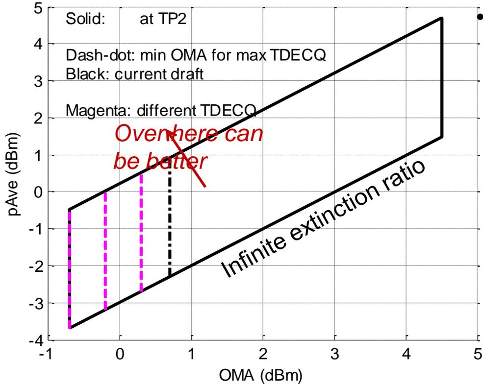
Black polygon: Tx spec in D3.1, with 4.5 dB min. extinction ratio
