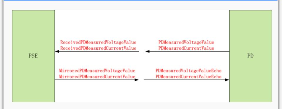
Note: The measured current from PD can be treated as a way for synchronization, since the current over the link segment is the same for PSE as well.
