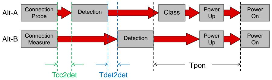
• Tpon: Ensures cable is not switched between end of detection and power on.
