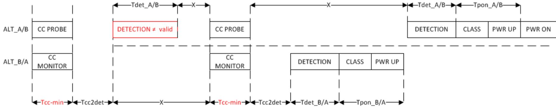
$T_{cc2det}$  is enforced for the first pairset to successfully power.
