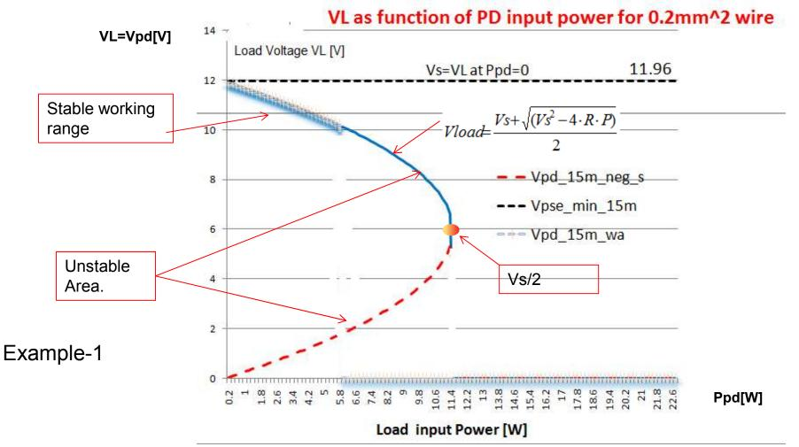
Plot of real system: load voltage vs. load power for 12V source (with 0.4Ω output DC resistance) for supporting 5-6W load
