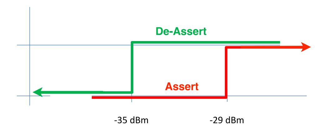
Assert function: Mandatory to "Sleep" -> "Wake up" at the threshold level at -29 dBm De-Assert function: Mandatory to "Wake up" -> "Sleep" at the threshold level at -35 dBm
