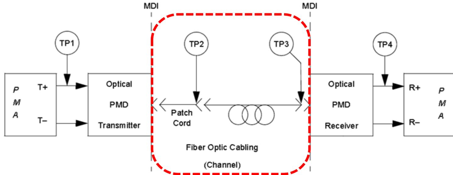
Scope of this presentation are the parameters from the optical link of the compliance points TP2 and TP3
