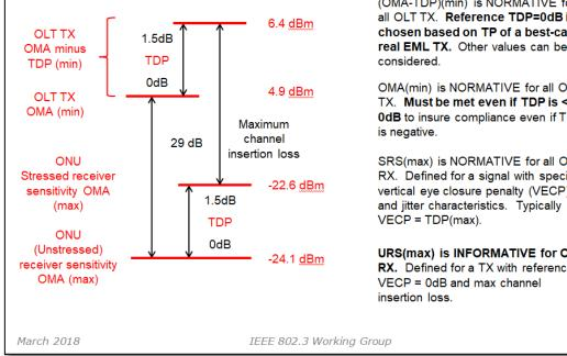
(OMA-TDP)(min) is NORMATIVE for all OLT TX. Reference TDP=0dB is chosen based on TP of a best-case real EML TX. Other values can be
