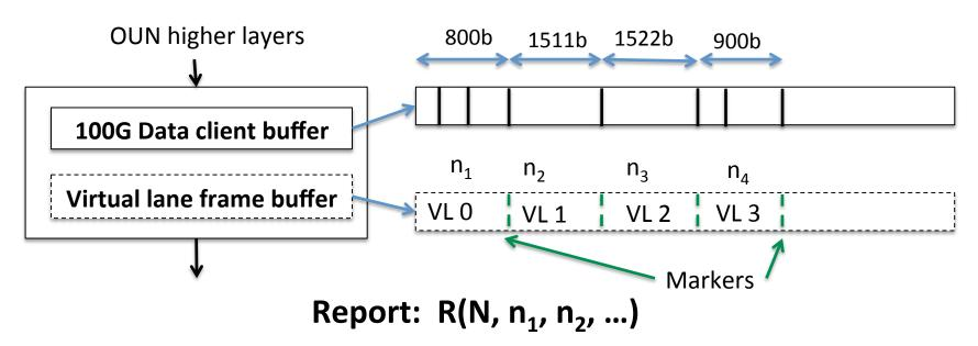
Where  $n_i$  (1  $\le$  i  $\le$  4) are frame boundaries for the close value of 1522 bytes\*. In above example,  $n_1 = 800$  bytes,  $n_2 = 1511$  byte,  $n_3 = 1522$  bytes,  $n_4 = 900$  byte. VL represent virtual lane. N is the number of lanes the ONU supports.
