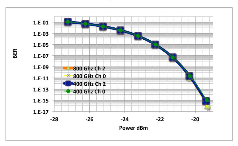
The BRE and power penalty performance of 400 GHz and 800 GHz uneven spacing channel plans and are almost indentical
