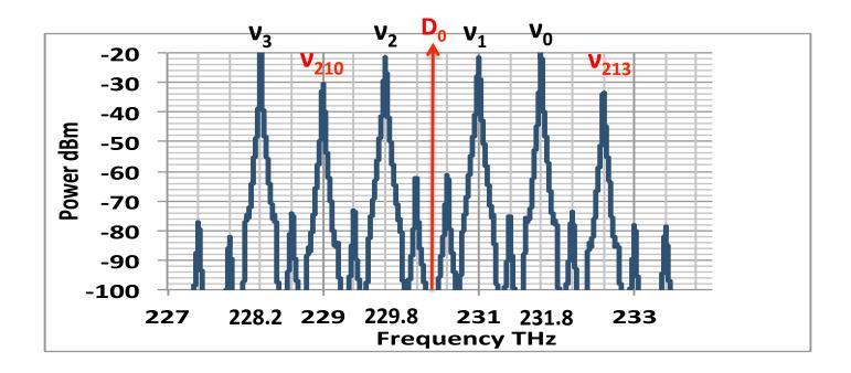
In this example of the worse case scenario of 4 channels 800 GHz uneven spacing DWDM with symmetric zero dispersion location, FWM mixing products  $v_{210}$  and  $v_{213}$  are strong but are out of band. If it were even channel spacing they would be in band under channel 3 and channel 0 respectively.
