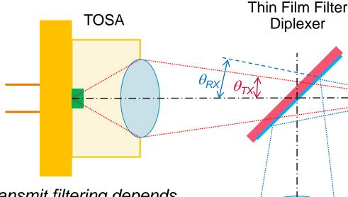
Transmit filtering depends on the TOSA beam width.
