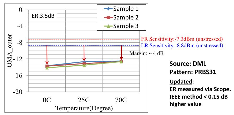
Margin >4 dB against -8.8 dBm LR (unstressed) receiver sensitivity spec for perfect transmitter (SECQ = 0dB)
