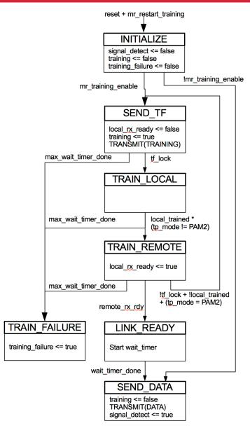
802.3cd D1.0 Figure 136-7 – PMD control state diagram
