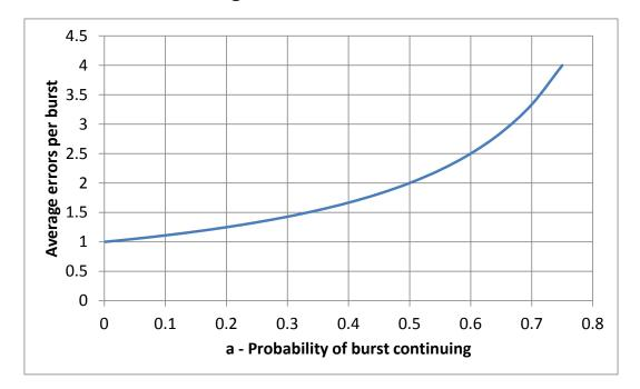
For a = 0.75, the BER<sub>in</sub> including bursts is 4 x the BER<sub>in</sub> due to noise.
