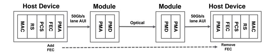
Then the worst case input BER for the FEC decoder must be met by the concatenation of all of the sub-links.
