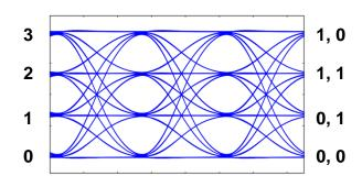
Since two of the eight possibilities result in both bits being correct, these states terminate the burst. Therefore for Gray coded PAM4, if a **symbol** is in error, the worst case probability that the next **symbol** is also in error is 0.75.
