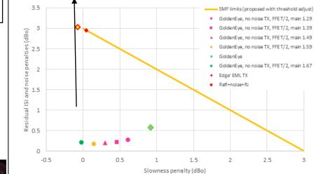
To emulate distortion, a reflection was added at 6UI -> TDECQ = 2.3dB. Added RJ (990fs) and noise (90uW, ≈1% signal strength) -> TDECQ = 2.95dB.
