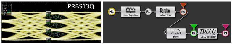
Using Keysight FlexDCA sim tool. Added 5T/2 TX Fir over GoldenEye <u>shared</u> waveform (kept PRBS13Q for faster processing), random Noise/Jitter block and 4th order BT filter.
