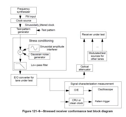
'The low-pass filter is used to create ISI. The combination of the low-pass filter and the E/O converter should have a frequency response that results in <u>at least</u> half of the dB value of the stressed eye closure (SECQ) specified in Table...'
