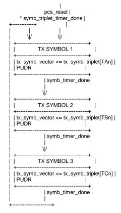
[7] Add text to subclause 146.3.3 'PCS Transmit' that reads 'The PCS Transmit function shall conform to the PCS Transmit state diagram in in Figure 146-5 and the PCS Transmit multiplexor state diagram in 146-6, and their associated state variables, functions, timers, and messages.'
