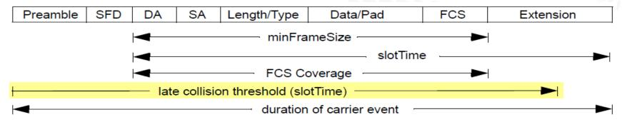
Figure 4–5—Frame with carrier extension
