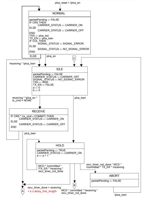
Figure 148-4—PLCA DATA state diagram
