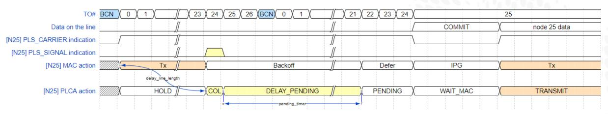
Collide and defer transmission when the maximum length of variable delay line is reached.
