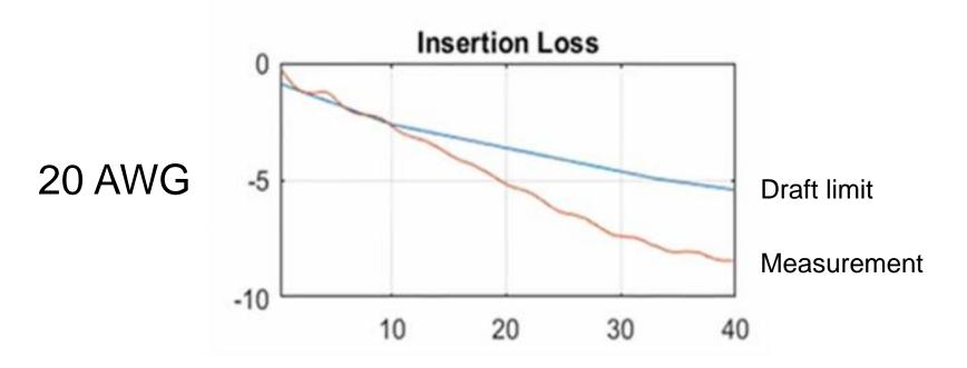
A number of cables were constructed and found to have more insertion loss than allowed, especially at high frequencies
