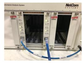
1 km balanced single twisted-pair 18 AWG 10 inline connectors
