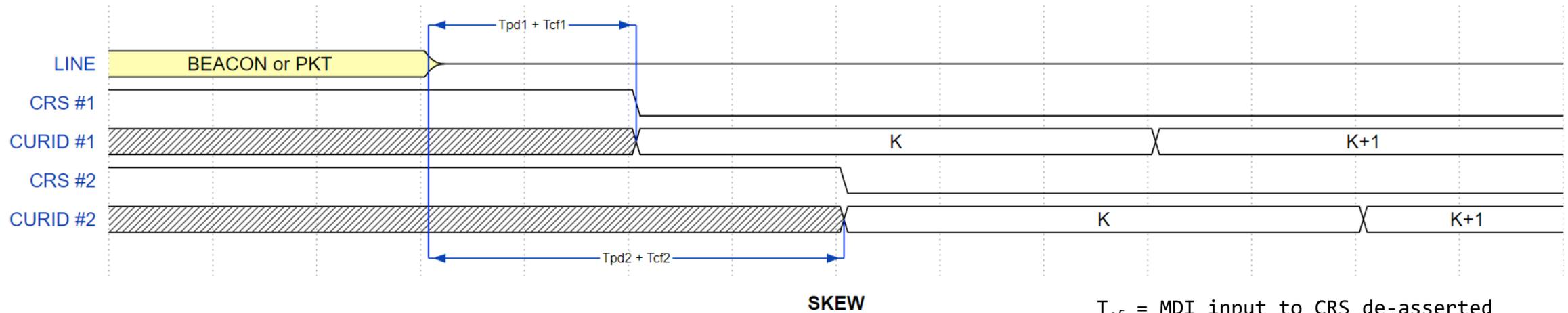
$T_{cf}$  = MDI input to CRS de-asserted
