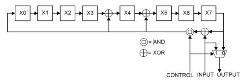
CONTROL = 1 when shifting the contents of the CLASS\_TYPE\_INFO register and calculating the CRC field
