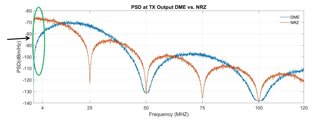
DME more spectrally compatible to automotive noise and PoDL than NRZ for 10BASE-T1S
