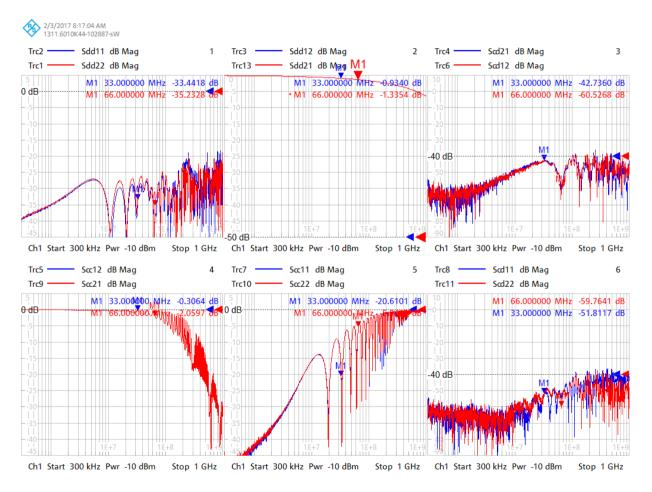
No unexpected nonlinear behavior for Sparameters below 1MHz
