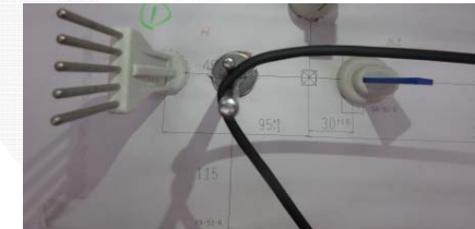
Figure 2: Bending on jig board
