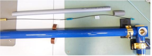
Coupling- and screening attenuation reference cable assembly
