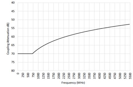
Figure 149–30—Coupling attenuation calculated using Equation (149–17)
