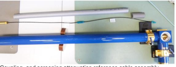
Coupling- and screening attenuation reference cable assembly
